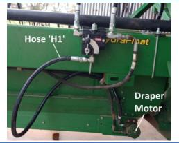
a) Connect the existing hose on the front coming from the return filter (hose AH227452) to the remaining end of the tee on the excess flow port of the flow controller.
