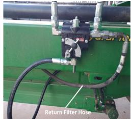
a) Ensure all connections are sealed and secure. Tighten any loose connections.
