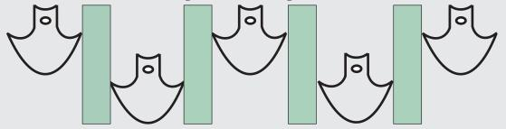
Coping with this problem by fitting wider points to compensate for progressive loss of overlap only means that for much of the points life fuel consumption is excessive and more soil is thrown than is necessary
