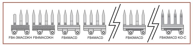
Right Hand Drive end Guards - 2 x FB40 MACDKH, then 2 x FB4 MACD, with trimmed upper ledger plates and or milled gullets to allow the knife heads adequate clearance. Wear strips are omitted for the same reason.
